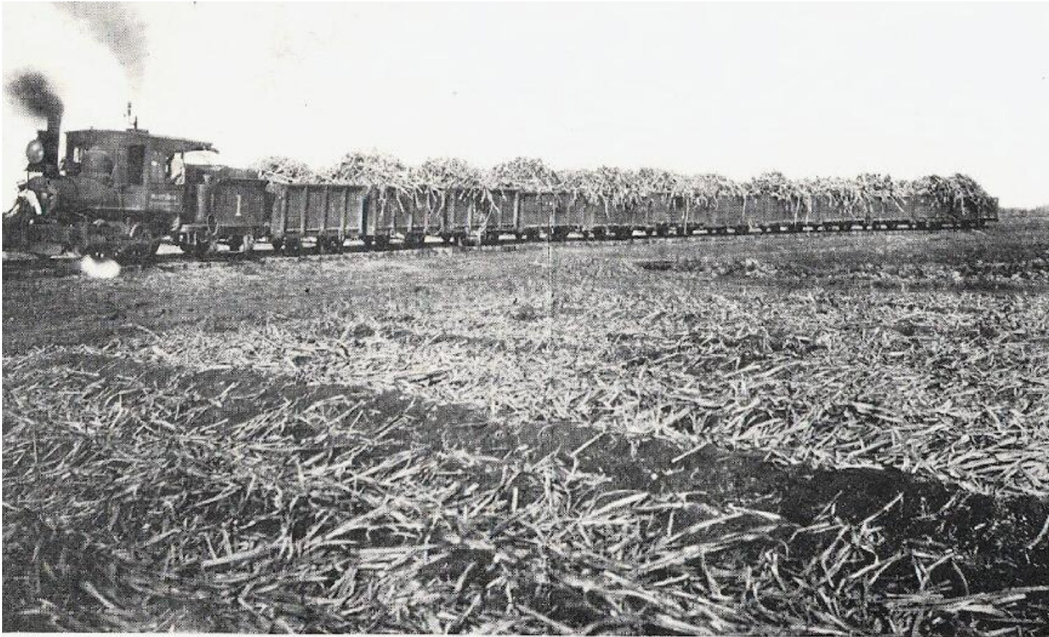
This is a narrow gage train in a sugarcane field in 1908 at Arcola Sugar Mills. This is a relatively small steam engine with only four drive wheels (two on each side) and no small steering wheels which are found on larger high speed engines. The light tracks were moved from field to field as the crops were rotated.
